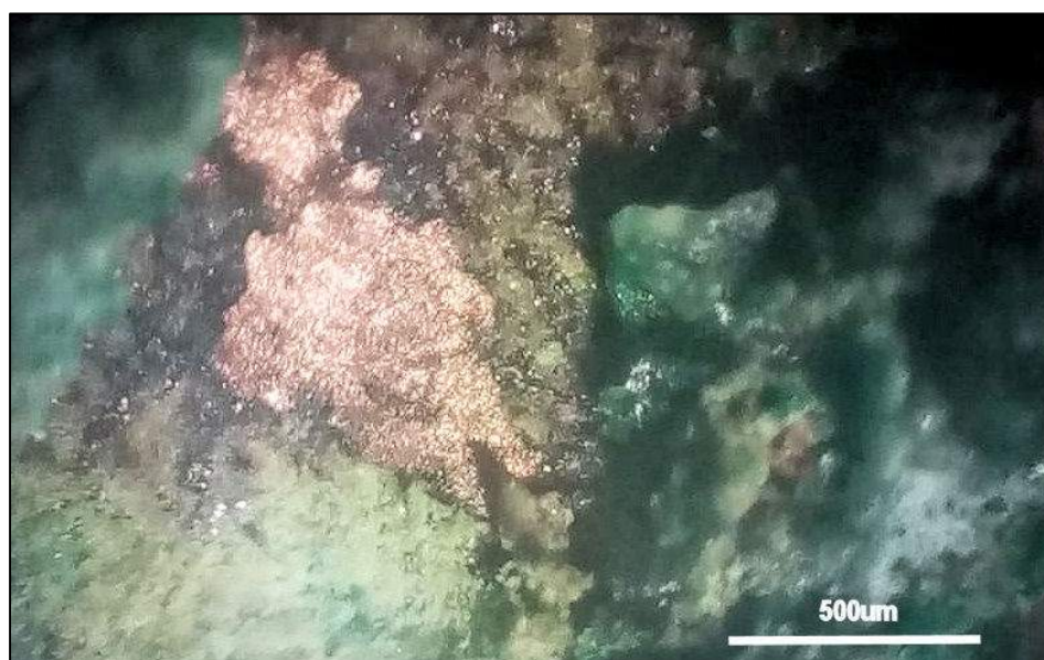
Figure 220. Photomicrograph of SF867, showing area of gold gilding under copper corrosion.
